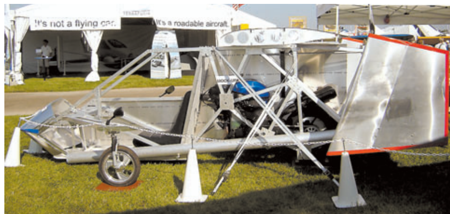
The mock-up model of the single-seat roadable aircraft Caravella Aerospace is developing at the 2008 EAA AirVenture exhibition in Oshkosh, Wis.
